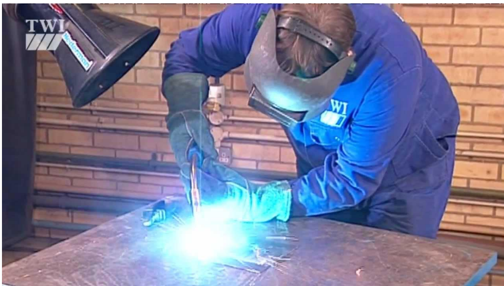
Figure 32. Arc welding showing PPE needed against UV and thermal radiation
