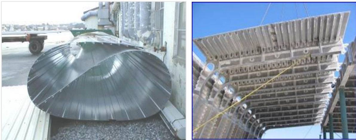
Figure 14. Rolled deck panel, left, and pre-fabricated hull module, right, both manufactured in aluminium by friction stir welding.
