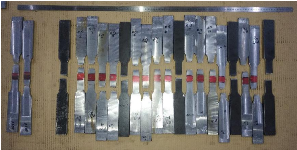
Figure 26. A friction stir weld in 12mm thick S460 steel sectioned and submitted to cross weld tensile testing.
